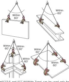
\*SCC0.5 and SCC-W(Wide Type) can be used only for vertical lifting, and use for lateral lifting is prohibited. SCC0.5 can be used for lateral lifting only by using a long shackle for SCC0.5 (sold separately).
