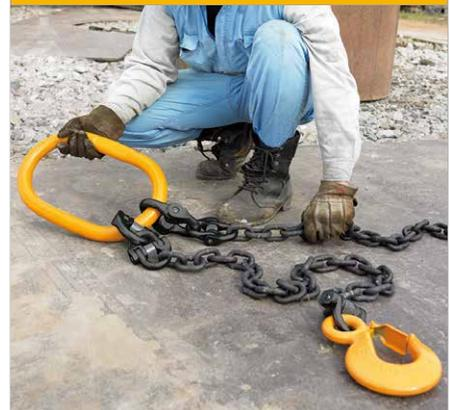
In the case of assembling set products using the Large Master Link HMG/HMH, use in combination with hi-couplings as described in the contents of the table at left.
