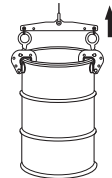
Vertical lifting is possible when DLC is combined with the balance for drum lift clamp.
