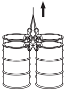
Lifting four drums with four clamps (in this case, the drums are lifted vertically.)
