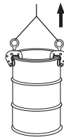
Using two clamps (This is safe when lifting a heavy drum, containing, for example, iron powder.)
